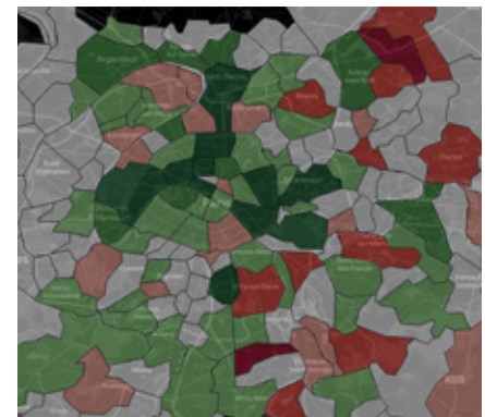
Change in mobile data traffic levels in the Paris area two weeks before and after lockdown in mid-March, showing a geographical shift in demand from central to adjacent and suburban areas
